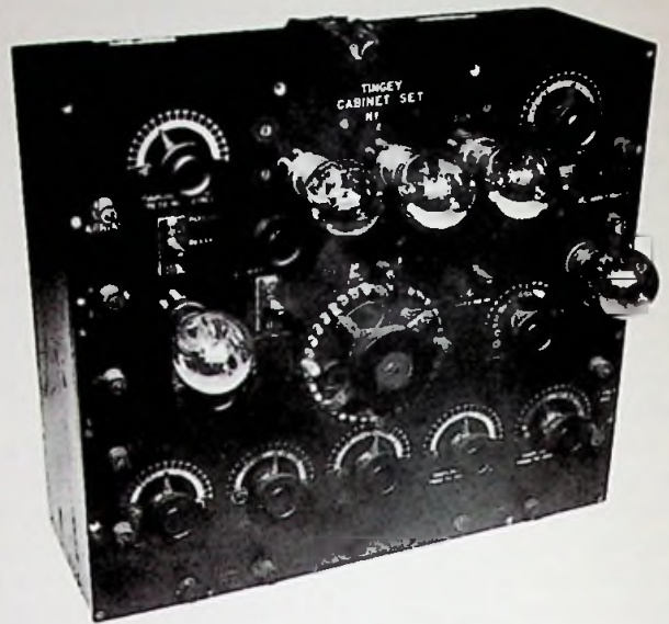
fig. 41. 'Cabinet Set', by W.R.H. Tingey. Early 1922. A 5-valve receiver with 3 or 5 valve switching, covering 175 to 28,000 metres in 7 stages, ebonite control panel, ebonised wood case. 16 in. x 18 in. x 7 in. Typical of the "fearsome" type of valve receiver described by Wireless World , with its scientific-looking panel bristling with controls.
