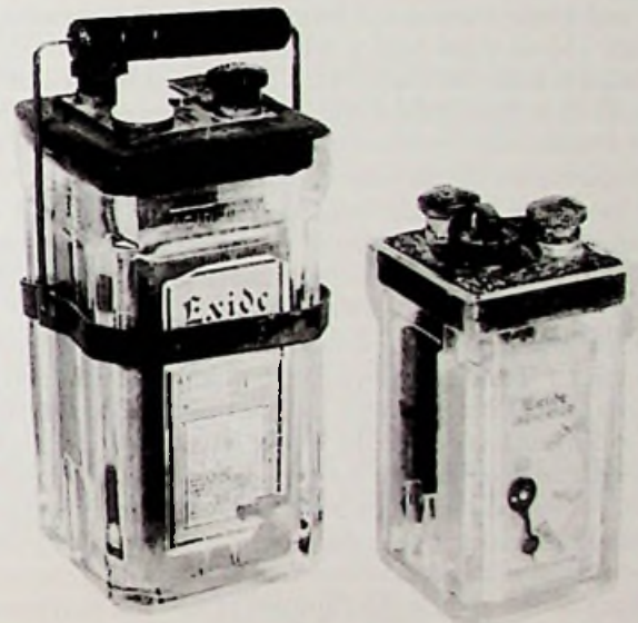
fig. 43 . Lead-acid accumulators, also known as 'LT' (low tension), 'secondary', 'storage' or 'wet' batteries, were re-chargeable 2 volt batteries of varying current capacity, consisting of a thick glass container in which two sets of lead plates were fitted. The plates were made up of lead grids filled with paste: a mixture of red lead, litharge and sulphuric acid for the positive plate, and a mixture of litharge and sulphuric acid for the negative plate, (the sulphuric acid in both mixtures was allowed to dry out before the cell was assembled). The plates, separated by hard wood or ebonite separators, were immersed in an electrolyte comprising a solution of pure sulphuric acid diluted with distilled water to the required specific gravity. Accumulators provided the filament current for the valves and would last about two to three weeks before they needed re-charging, depending upon the number and the type of valves used and the time spent 'listening-in'. In 1922, a 3-cell 6v accumulator of 40 ampere-hour capacity complete in a 7¼ in. x 10 in. x 5½ in. wooden carrying crate cost around £2.10s.0d, and the re-charging service, which usually took about 24 hours, cost around 6d. From the mid-1920s, 'unspillable' accumulators with a 'jelly' electrolyte and accumulators housed in lighter weight 'unbreakable' celluloid containers became popular for use with battery portable receivers. The LT batteries in the photograph date from the late 1920s.
