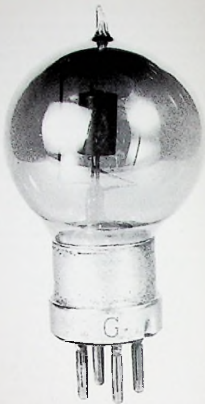
fig. 38. 'R' Valve (actual size), by British Thomson-Houston Co. Ltd. Late 1922. A bright-emitter with a nickel-plated base. 4 ¼ in. high. Etched with the BBC/PMG stamp.
