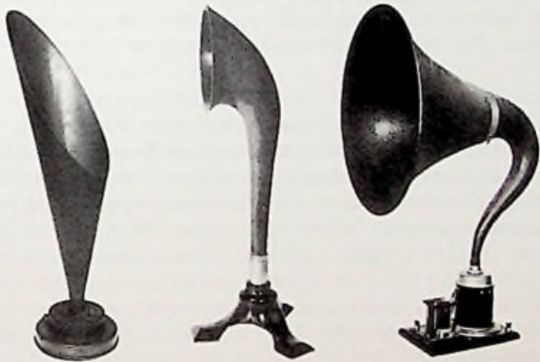
fig. 42 . Straight-necked, curved-necked and swan-necked horn loud-speakers of 1922.
