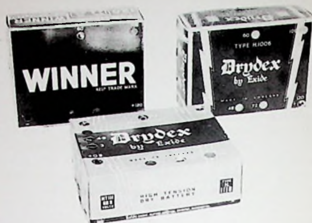
fig.44 . High tension ('HT') batteries, which were also known as 'primary' batteries, were necessary to provide the valves with anode voltage, and comprised a large number of series-connected 1½ volt dry cells usually arranged neatly in a strong cardboard box and well sealed in with paraffin wax or pitch to form a single unit. Depending on the valves and the type of receiver used, HT batteries in sizes from 45 volts to as much as 180 volts were available, and these were provided with tappings taken from groups of cells at regular intervals so that variations in voltage could be obtained as desired. While being non re-chargeable, a good quality HT battery could, with average use, last for about three to four months and in 1922, one of 60 volts in a 3½ in. x 9 in. x 2¾ in. container cost around £1.0s.0d. HT batteries were sometimes made up of series-connected accumulators, but these were usually used only by listeners who were in a position to do their own re-charging or had a regular collection and re-charging service. The HT batteries in the photograph date from the 1930s.
