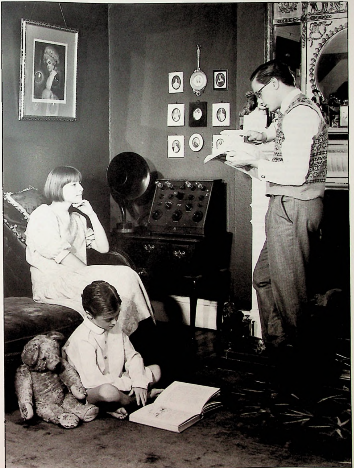
A.J.S. 4-valve battery receiver, 1923, with an S.G. Brown Model H1 horn loud-speaker.
