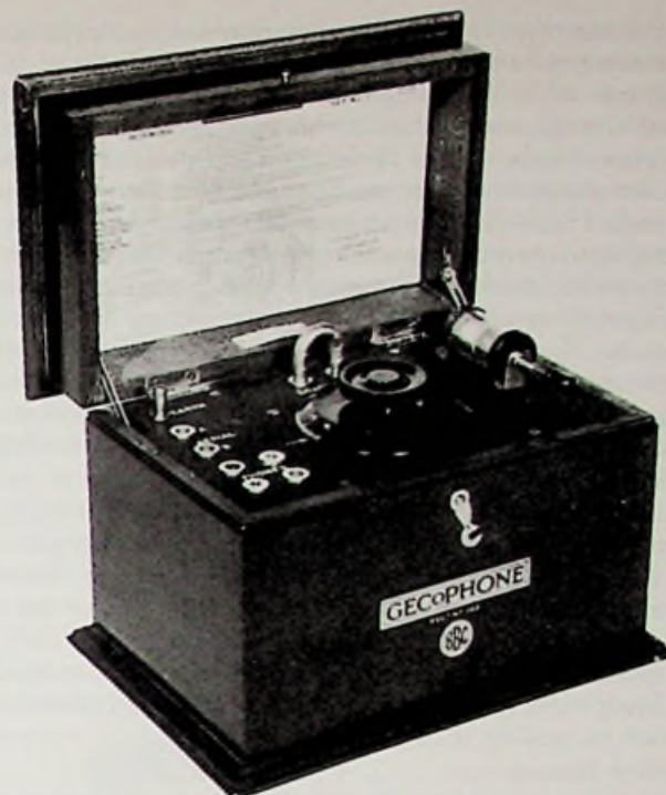
fig. 39. Gecophone Model No.1 Type BC 1002, by General Electric Co. Ltd. 1922. BBC/PMG Stamp, GPO Reg.No.102. Crystal set for headphone use, glass-enclosed cat's whisker/galena detector (open detector version also known), provision for plug-in coils, variometer tuning, ebonite control, nickel-plated fittings, mahogany box with lift-up lid. 6 1/4 in. x 9 in. x 6 in. (closed). £5.10s.0d.
